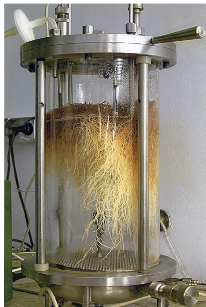
Fig. 6 P. grandiflorum hairy root biomass of transgenic line PI 17 after the culture period of 12 weeks in 5-l bioreactor with liquid WPM medium supplemented with 40 g/l sucrose.
